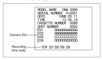
The details in the shot data depend on the shooting conditions. If because of the devices used there is no shot data on a part of the tape, it appears as blank.
