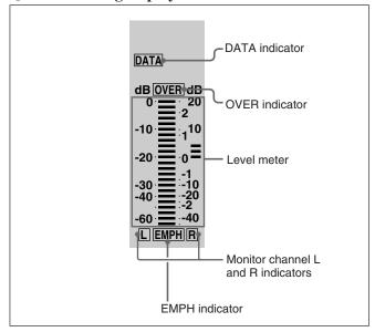
**DATA indicator:** Lights when the audio signals are recognized as data signals.
