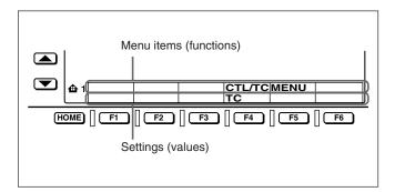
In the figure above, TC (time code) is selected as the setting for CTL/TC (time data selection), the menu item for button F4. This manual refers to this as "F4 (CTL/TC) in function menu HOME page is set to TC."
