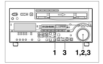
1 Press the SHUTTLE button or search dial so that the SHUTTLE button is lit.
