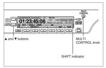
When the menu item number displayed in the menu display is flashing, you can change the menu item by turning the MULTI CONTROL knob.
