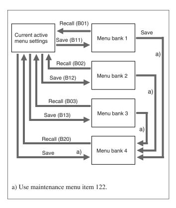
The current active setup menu settings as well as settings saved in menu banks are stored in separate storage areas for 59.94i, 29.97PsF, 23.98PsF and 50i, 25PsF, 24PsF modes.
